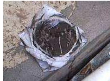
**Figure 18** Contamination residue on the first-flush cloth filter
